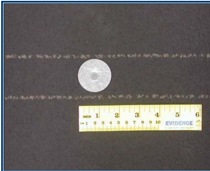
Photo 2: View of Nail & Tin-Cap Specimen
